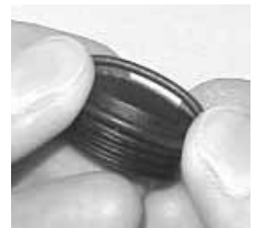
Fig. 98 - INSTALLING THE COVER O-RING
